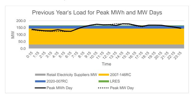
Peak MW occurred on 13:15 of May 16, 2019 due to load behaviour of BATELEC II. Peak daily MWh occurred on 14:15 of June 4, 2019 due to load behaviour of BATELEC II. As shown in the Load Curves, the available supply is lower than the Peak Demand.
