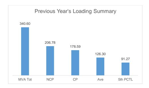
The Non-coincident Peak Demand is **206.78** MW, which is around **63.59%** of the total substation capacity of **340.6** MVA at a power factor of **0.9547**. The load factor or the ratio between the Average Load of **126.30** MW and the Non-coincident Peak Demand is **61.08%**. A safe estimate of the true minimum load is the fifth percentile load of **91.27** MW which is **44.14%** of the Non-coincident Peak Demand.
