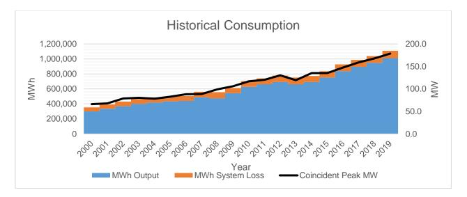
MWh Output **decreased** from year **2012** to year **2013** at a rate of **4.59**%, while MWh System Loss **increased** at a rate of **4.98**% within the same period.
