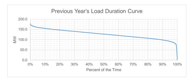
Based on the Load Duration Curve, the minimum load is **14.497** MW and the maximum load is **178.592** MW for the last historical year.
