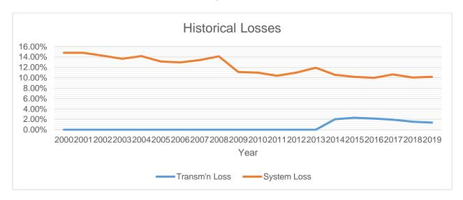
Historically, Transmission Loss ranged from 1.39% to 2.31% while System Loss ranged from 9.99% to 14.82%. Transmission Loss peaked at 2.31% on year 2015 because it was the first whole year transition period of BATELEC II with customer under Retail Electricity Supplier (RES). System Loss peaked at 14.82% on year 2000 because of not enough system loss reduction projects were planned and executed.
