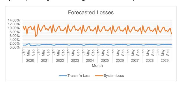
Transmission Loss is expected to range from **0.84**% to **1.86**% while System Loss is expected to range from **5.63**% to **11.93**%.
